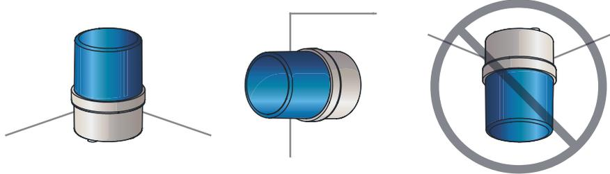
※ For products with a protection rating of less than IPX4, please install it vertically.
